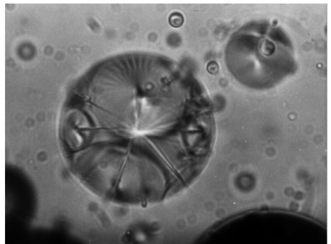
Figure 1. SmecticA Focal Conic Domain obtained by conventional light microscopy.
