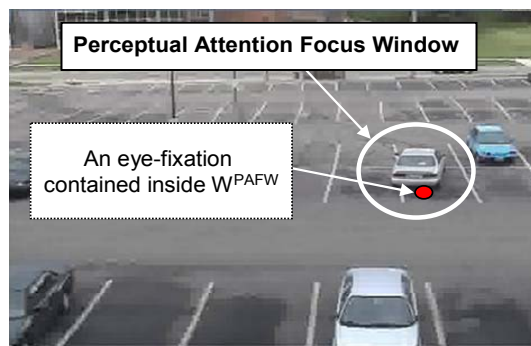
Figure 4. “Car” video. The frame is compressed from 10Mb/s to 1Mb/s based on the PATf concept. The eye-fixation is contained inside of the W^{PAFW} .
