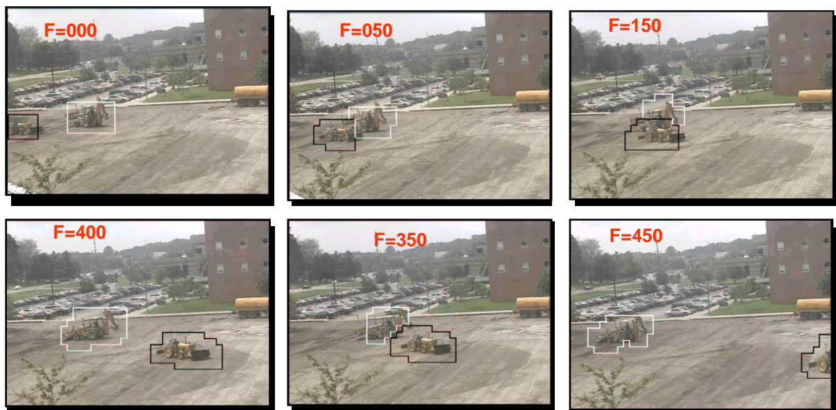
Fig-4. Results from tracking two objects simultaneously. The figures shows the boundary of the active block sets at 50 frame intervals. FOB algorithm tracks objects in P & B frames with reverse extrapolation on I frames.
