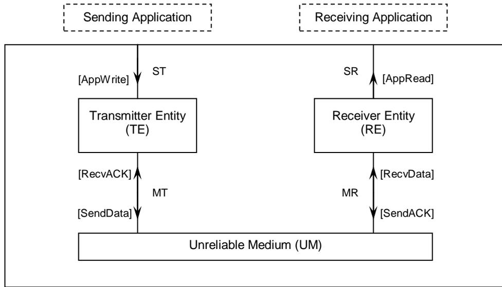
Figure 11. Simple TCP system composition
