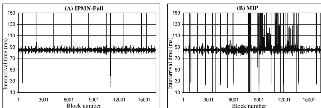
Figure 34. Block interarrival times at the MN (Jitter)
