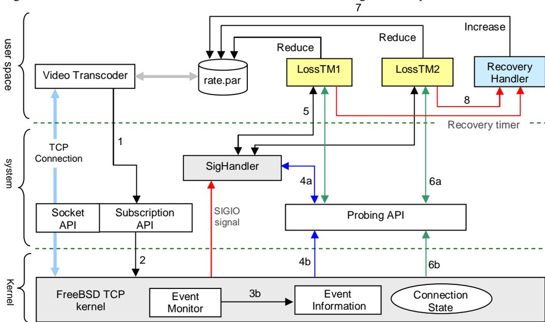
**Figure 16. The TCP-interactive extension and API**
