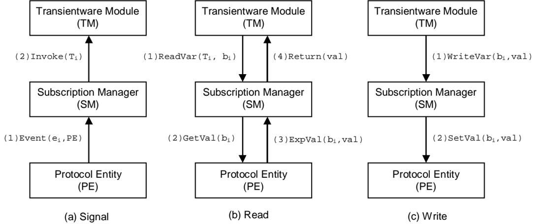
Figure 5. Interfacing between the PE and the TM
