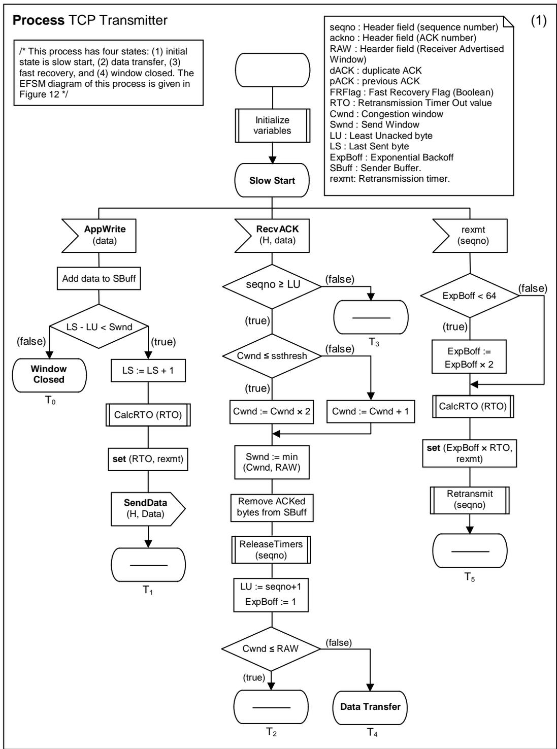
Figure 14. SDL description of a simplified TCP transmitter
