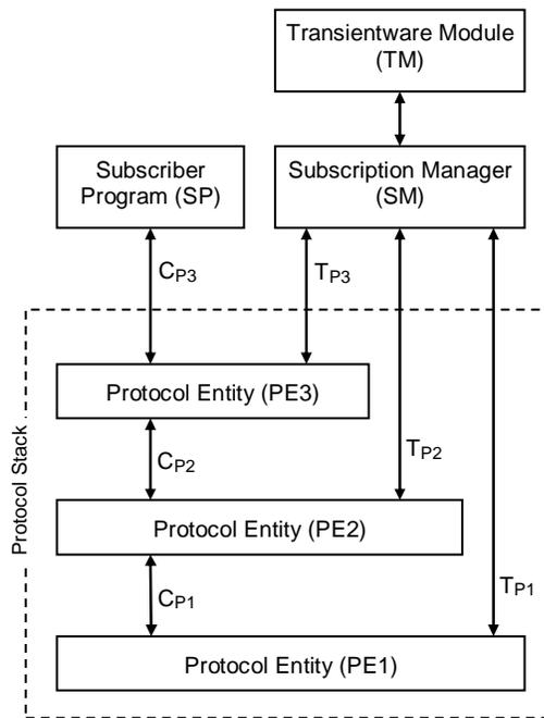
**Figure 2. *T*-type channel extension**
