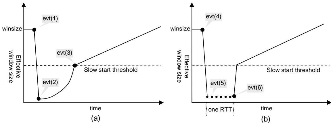
Figure 10. Changes on TCP's sending window due to congestion control events
