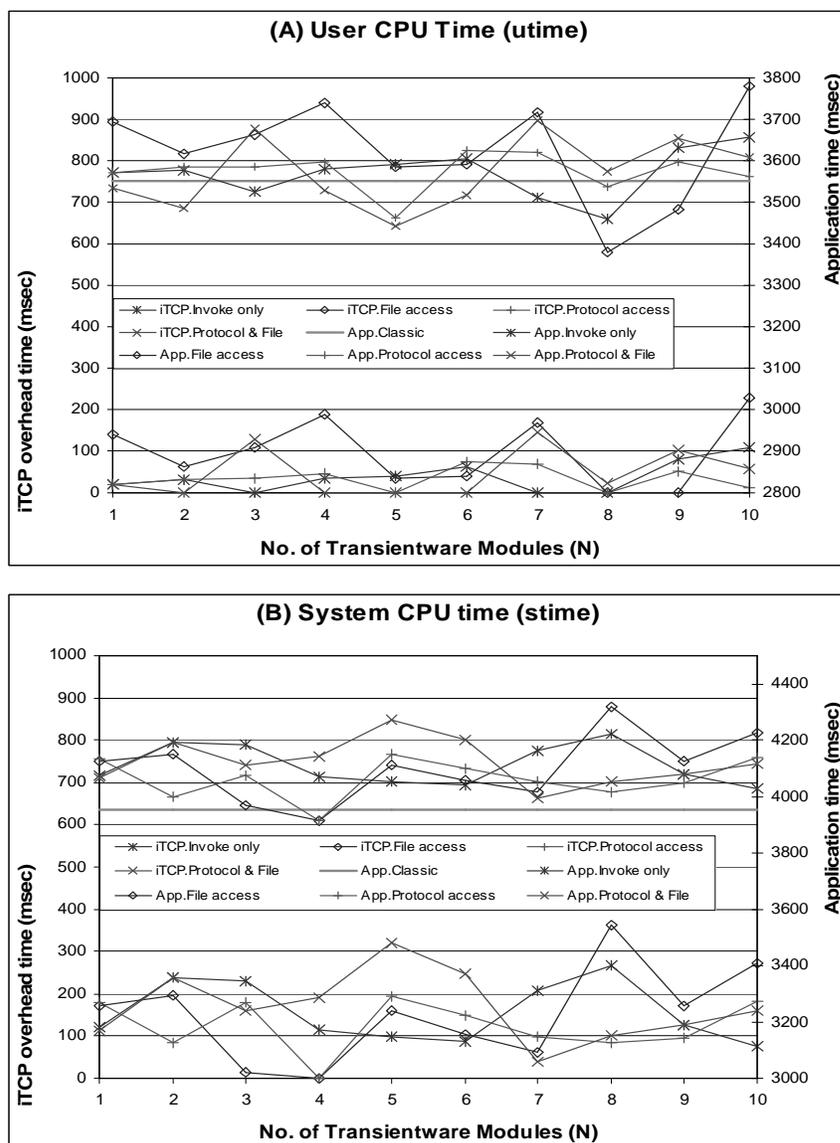
**Figure 41. iTCP CPU time overhead**
