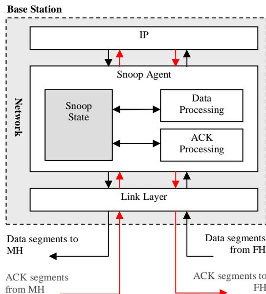
Figure 37. Conventional Snoop mechanism
