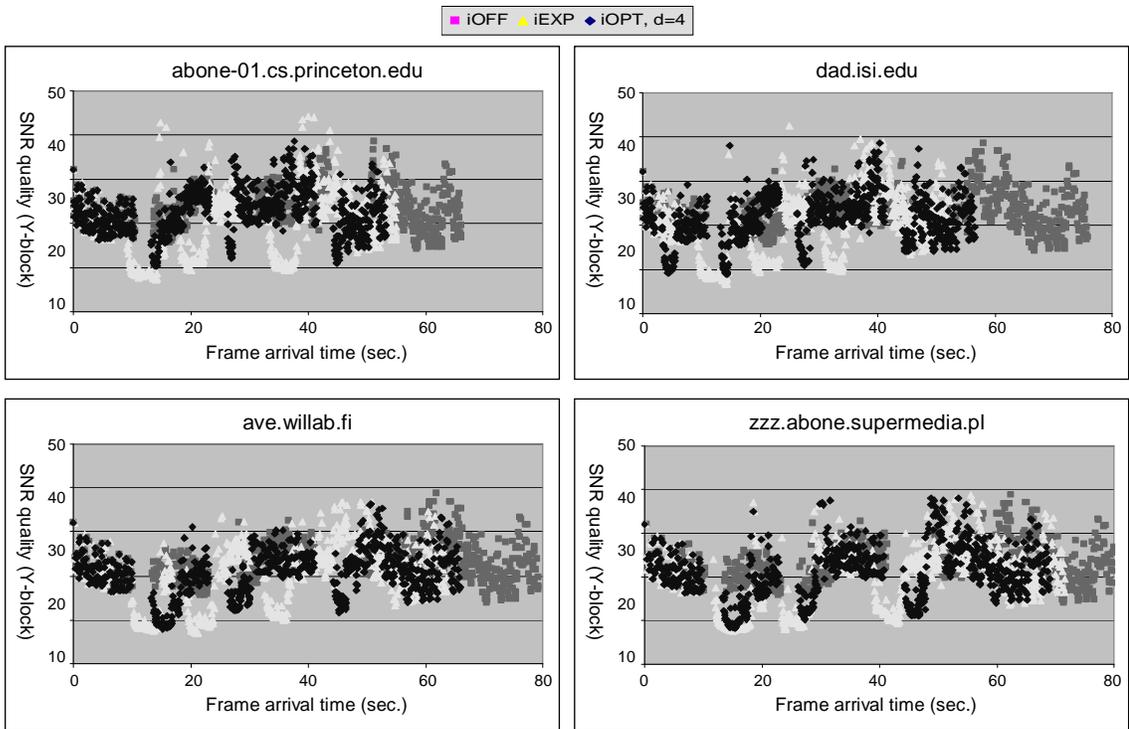
Figure 26. Frame Arrival time and frame SNR quality tradeoff
