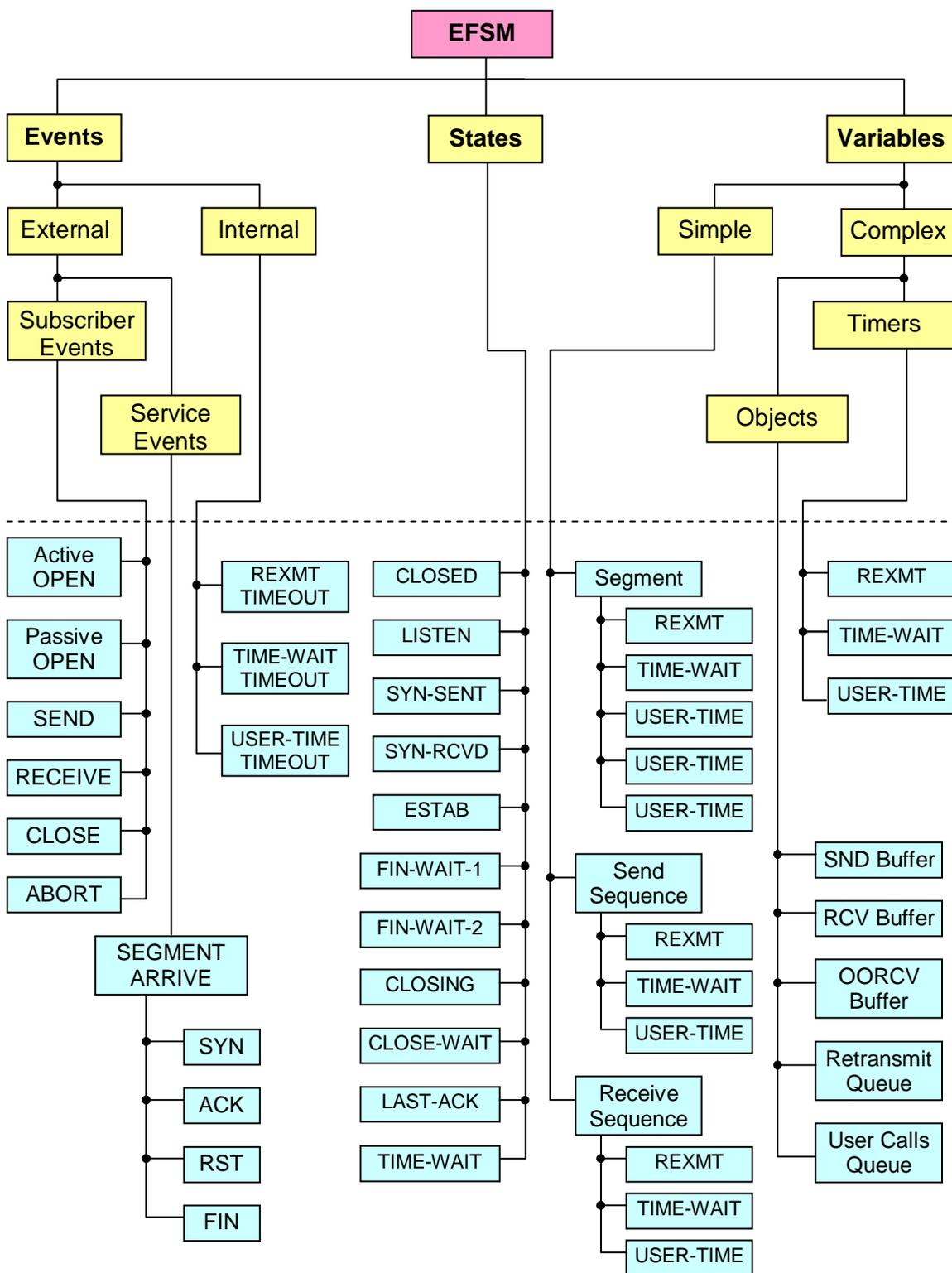
Figure 13. Classification of the EFSM components and their TCP counterparts
