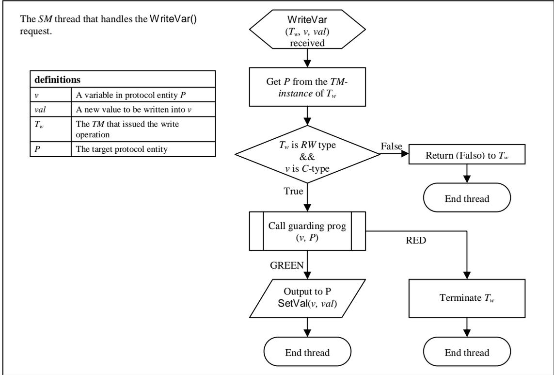
**Figure 7. *SM* handling of the `WriteVar()` operation**
