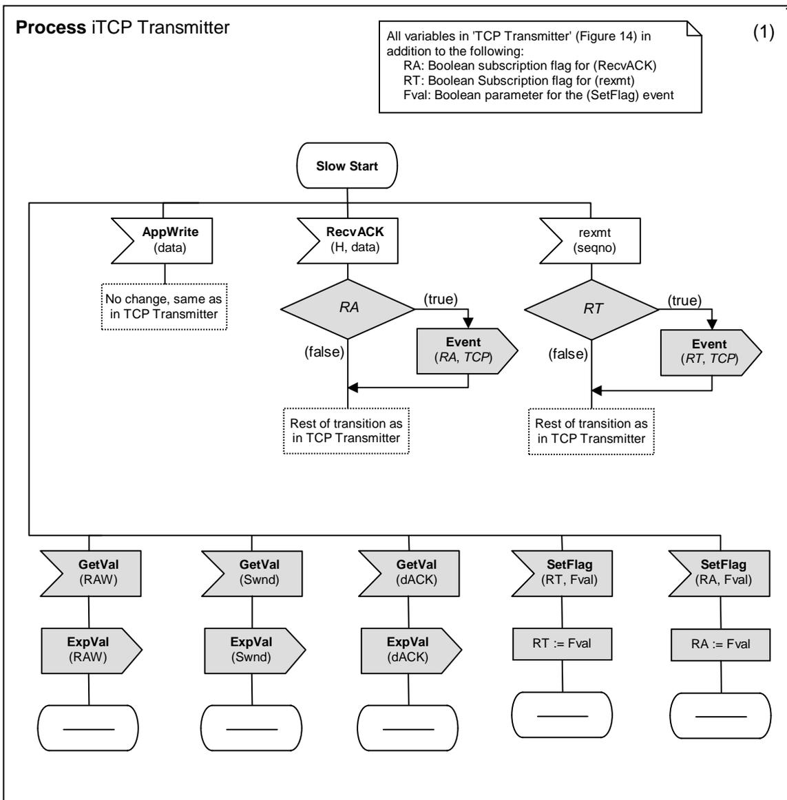
Figure 15. iTCP's (Slow Start) state extended with *InTraN* components
