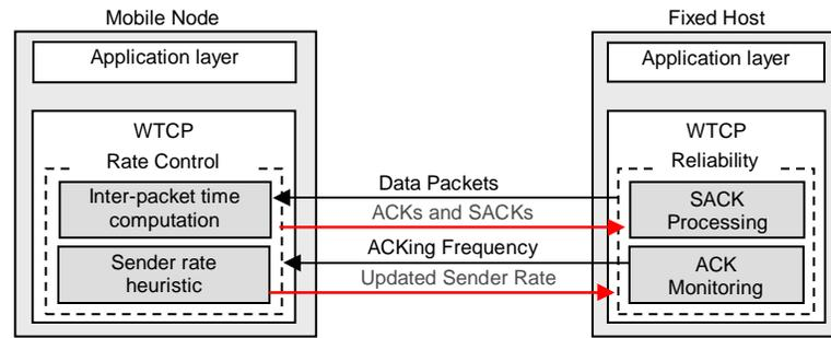
Figure 39. Conventional WTCP mechanism
