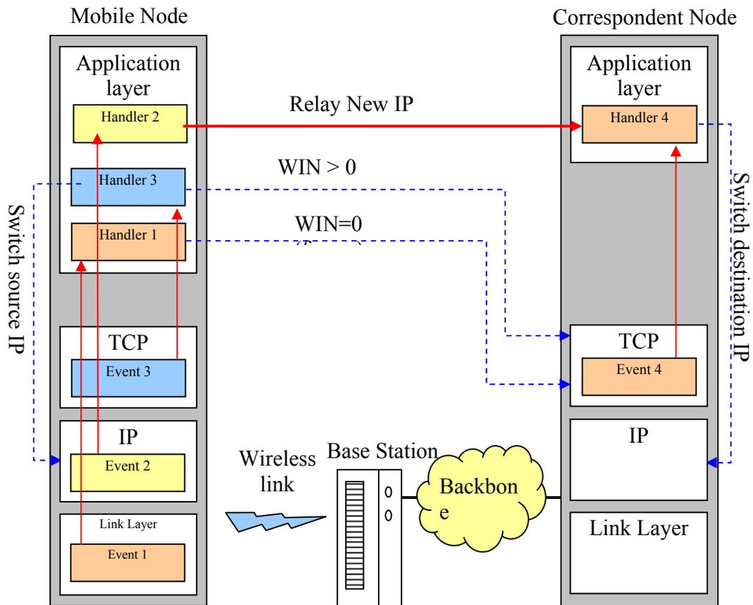
**Figure 4. IPMN-Half architecture and event sequencing.**
