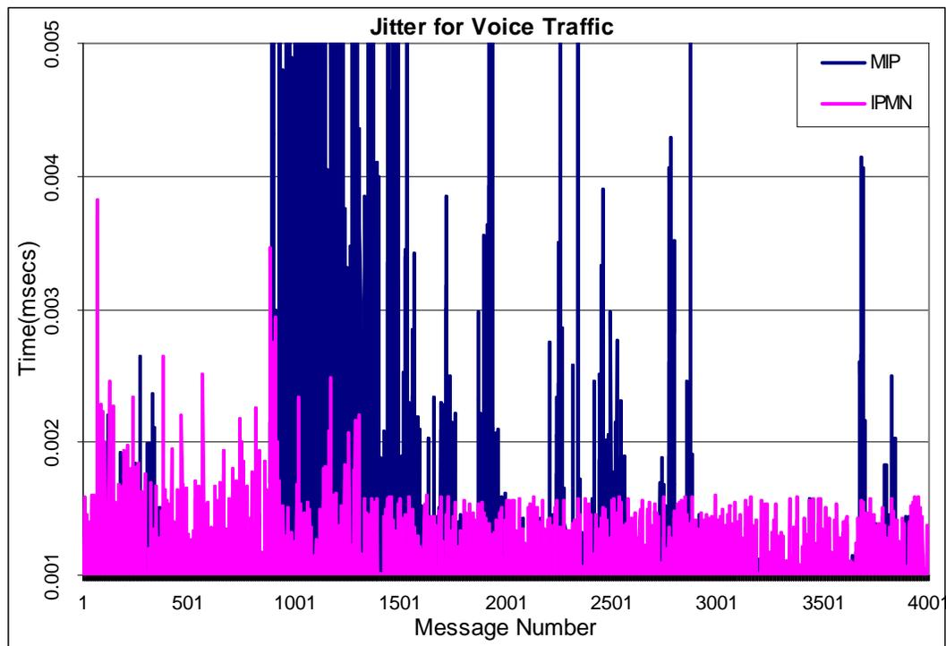
**Figure 22. Jitter In Voice Traffic with Voice Cross-Traffic.**
