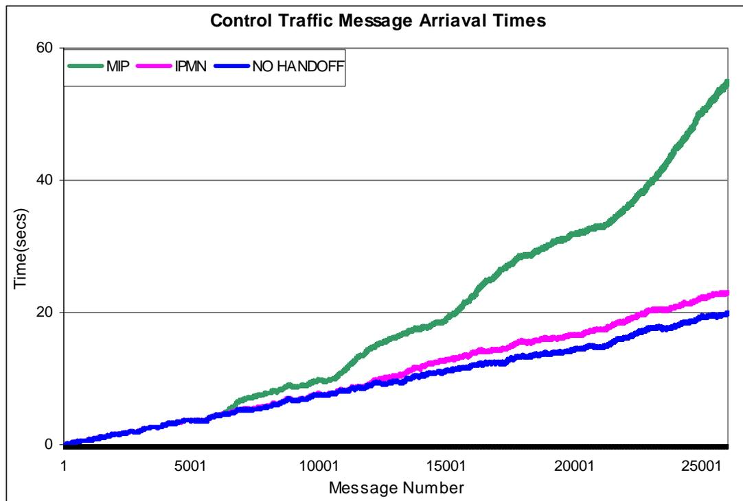
**Figure 25. Control Traffic Arrival Times with Random Cross-Traffic.**
