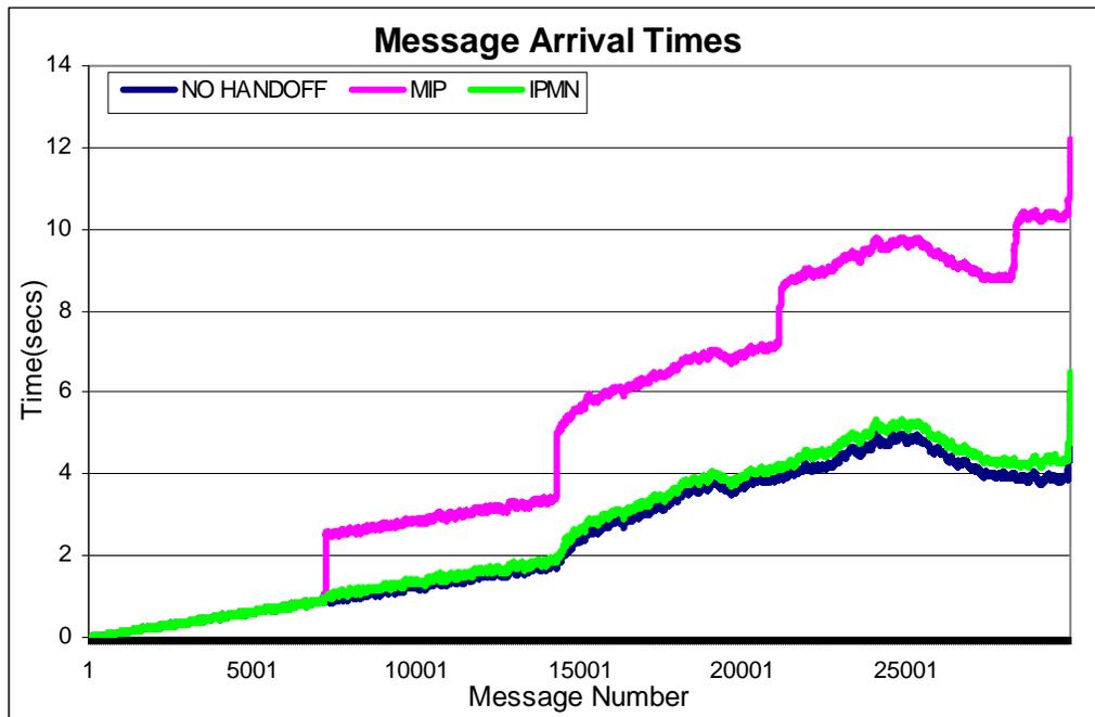
Figure 19. Message Arrival Times with 10% BER and FTP Cross-Traffic.
