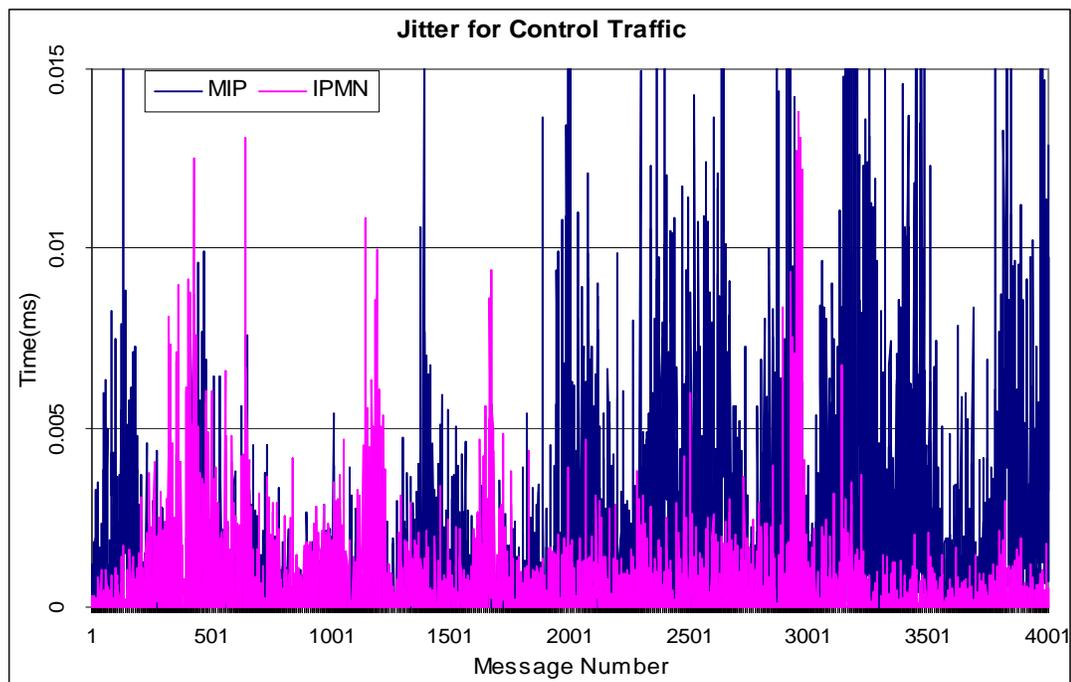
**Figure 26. Jitter in Control Traffic with Random Cross-Traffic.**
