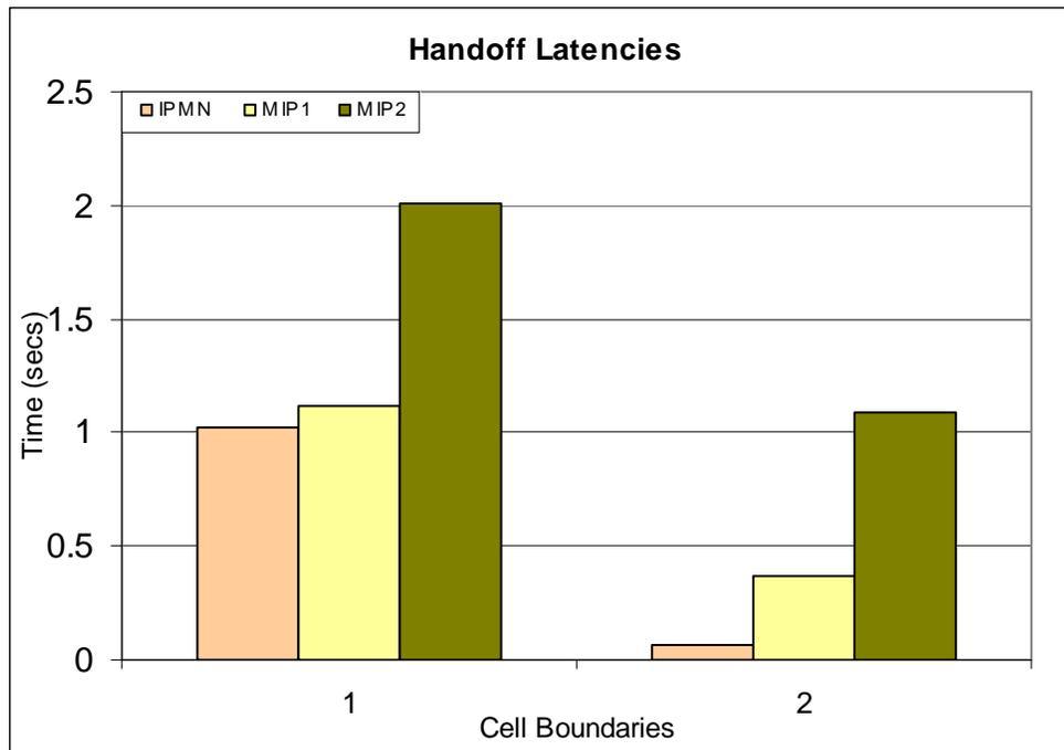
**Figure 17. Handoff Latencies of Mobile IP and IPMN. MIP1 has a AA lifetime of 100ms and MIP2 1sec.**
