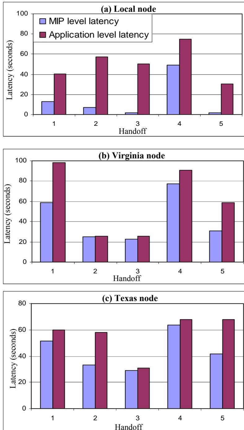
**Figure 9. Handoff latencies on both MIP level and application level.**
