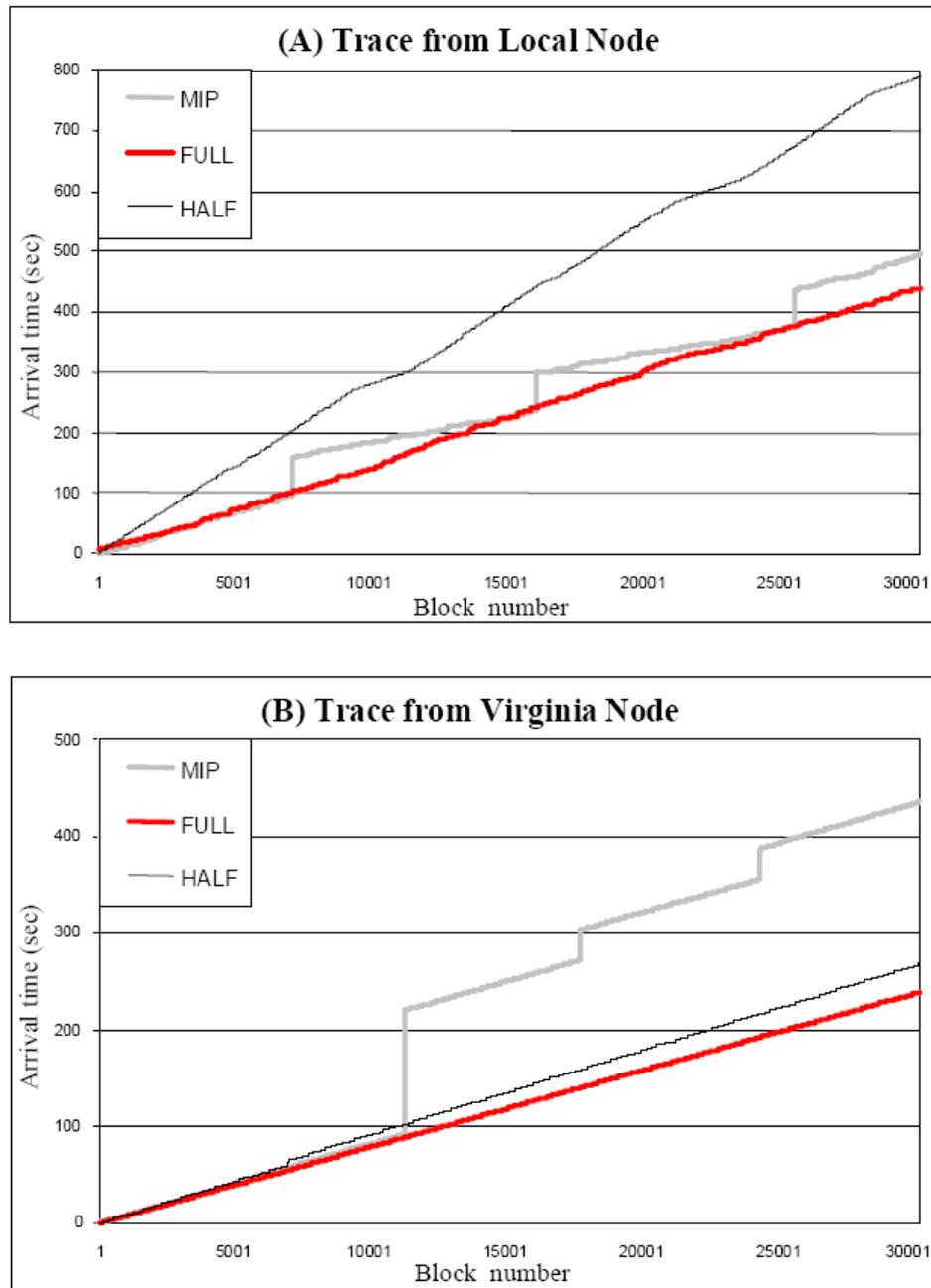
**Figure 10.** The arrival time of each 144-byte block (talk burst) at the MN from (a) Texas node and (b) Virginia node.
