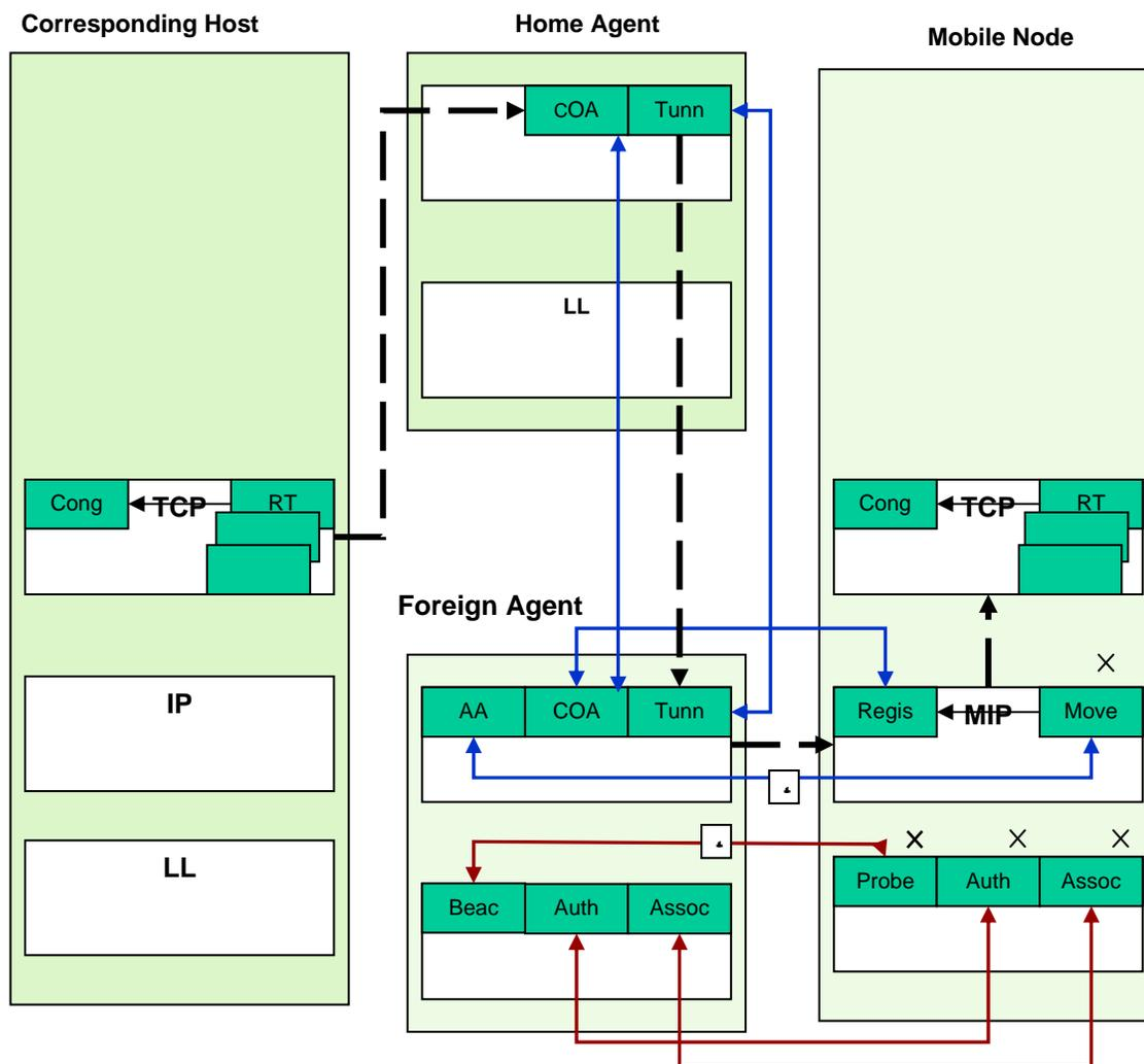
**Figure 1. Mobile IP's Complex Handoff Procedure.**
