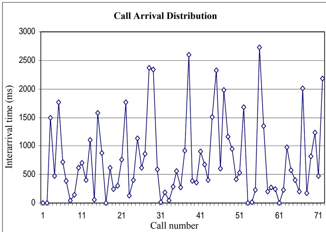
**Figure 6. Call interarrival sampling over 5 hours for  $\lambda = 1$  for Voice Traffic.**
